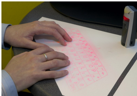
Figure 2.7: Celluon usage Example (Courtesy of Canesta Inc.)
