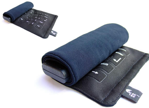
Figure 2.1: Bluetooth textile keyboard (Courtesy of Eleksen)
